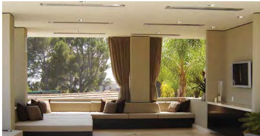
Contemporary outdoor room with W-Series heaters flush mounted into a drywall ceiling
