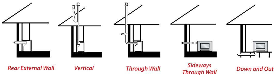
**Please note:** \*Suitable for direct, vertical or horizontal flueing. 500mm required for down and out applications. See installation instructions for full details.
