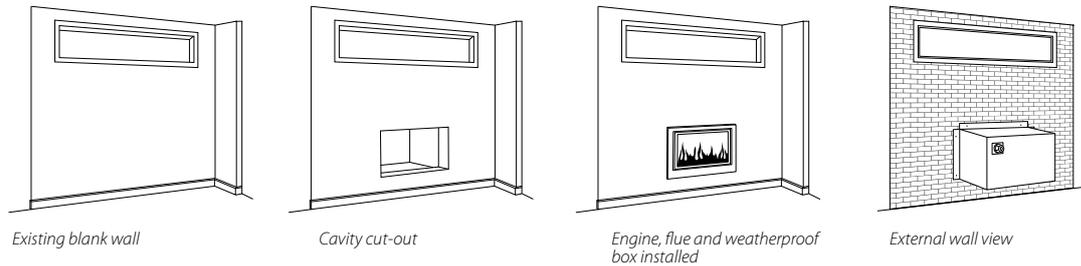
For an alternative installation to a false fireplace, the Rinnai 950X can be installed into a weatherproof box. A cavity is cut into the existing blank wall and the fireplace is installed onto a bracket that allows the back of the fire to sit outside housed in a tightly sealed box. This option allows the fire to be built into an existing wall without taking up any extra space in the room. The weatherproof box is sold separately.
